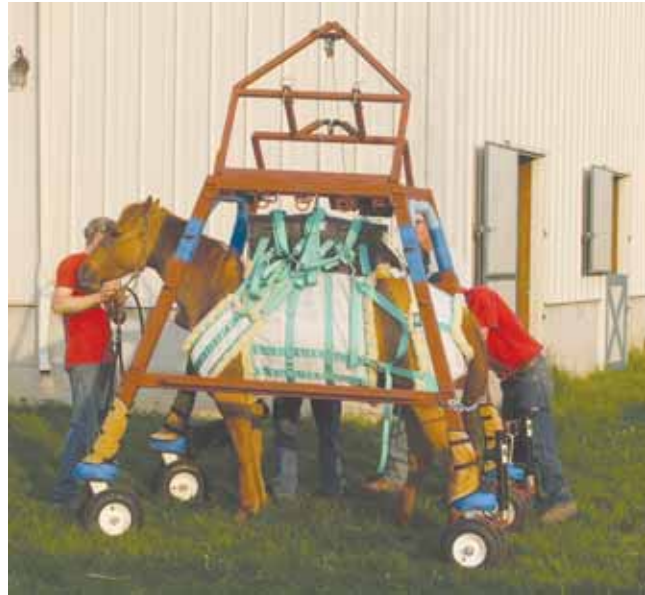
Fig. 1. The Falkner Walker h with support sling. This allows mobility and manipulation of the patient without fully loading the limbs.
