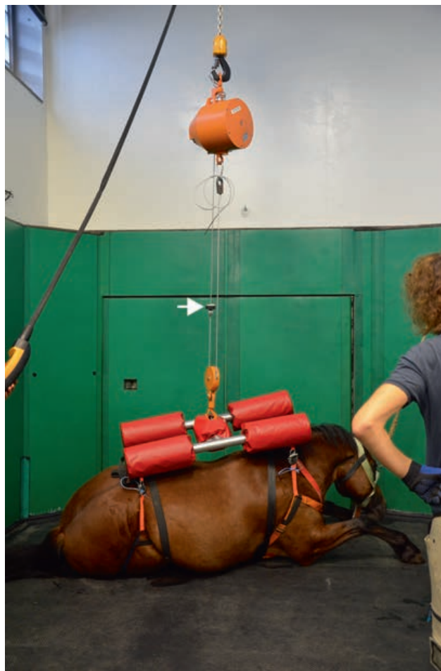
FIGURE 3 Balancer under full load indicated by the pulled-out balancer wire cable. Arrow: Mechanical cable-stop at the end of the balancer wire cable.
