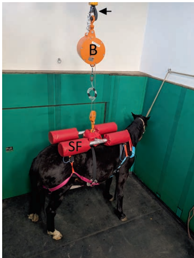
FIGURE 1 Balancer-assisted sling recovery system consisting of a sling in combination with a 4-point support frame (SF; red) and a balancer (B; orange housing). The balancer is connected between the hoist (arrow) and the support frame. The system is used in combination with a head rope.
