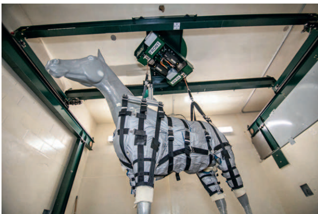
Fig 2: Equine rehabilitation lift and model horse used for initial testing to ensure material strength and safety. The computer-controlled lift, designed and built by RMD Engineering, Inc., and installed at the Western College of Veterinary Medicine (WCVM), allows for separate front- and hindlimb support (labelled as “Front” and “Rear”). A rehabilitation harness for use with the lift is under development, with one prototype shown here. Photo: Christina Weese (Foxtailstudio.net) for WCVM.
