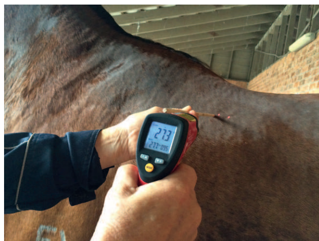
Fig 1: The hand-held infrared thermometer being used on the shoulder area of a horse for the prerace measurement. The baton is only used here to demonstrate the recommended distance of 30 cm, which corresponds to 2.5 cm between the laser dots. The horse must have a fine summer coat.
