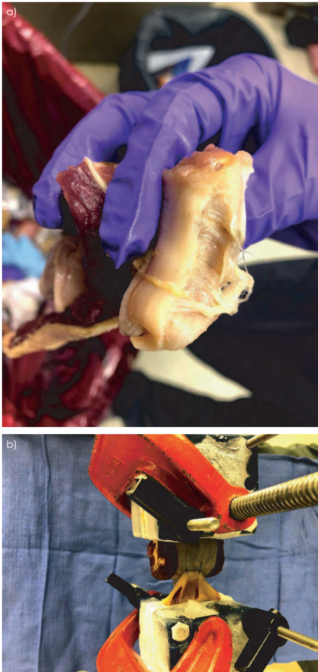
Fig 3: Failure of the colon wall at the suture site within the lateral band (a was predominant in samples harvested for ex vivo biomechanical testing of colopexy pullout strength b).
