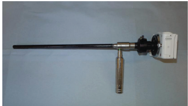
Fig. 10. Digital camera with wifi capability coupled to a rigid endoscope with a battery-operated LED light source. Pictured here is a Panasonic Lumix h GF6 camera with a micro four-thirds to C-mount adapter and a C-mount coupling lens. (Courtesy of Jack Easley.)
