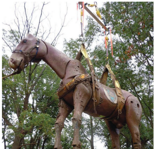
Fig. 13. Here students practice a vertical lift using the Becker Simple Web Sling and a crane. The mannequin is simulated to be sedated for this procedure to minimize struggling and possible injury to itself and handlers. The most dangerous times are at lift off and set down of the animal—when a live animal can get leverage and launch itself forward. Photo by permission.
