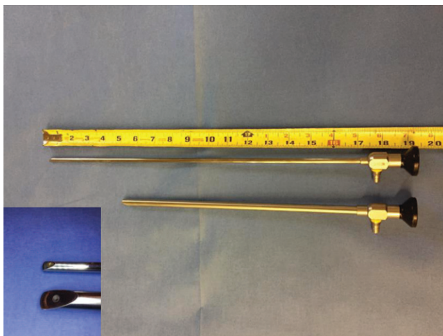
Fig. 6. Example of rigid endoscopes (Top, 6 mm × 30 cm and bottom, 10 mm × 42 cm) both with 70° viewing angles. (Author photos.)
