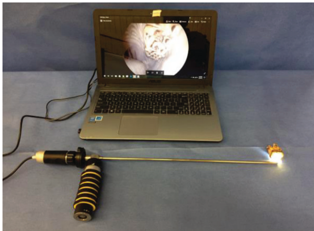
Fig. 9. USB camera mounted on a 6 mm × 42 cm 70° viewing angle scope with a battery-powered LED light source. (Author photos.)
