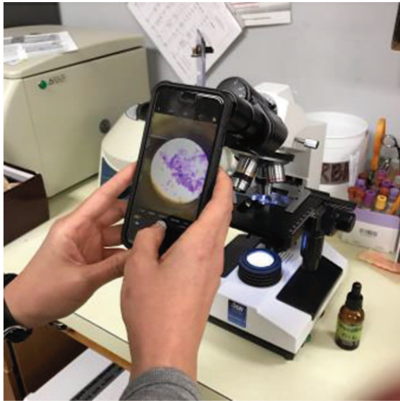
Fig. 20. The tiny lens of modern cell phone cameras easily captures excellent digital images of cytology samples. Most of the images in this paper were taken with an Apple iPhone camera through the microscope shown.
